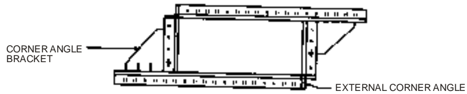
Fig. 5.6B : Two Sides Adjustable Column Form
