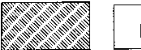
Fig. 7.4 : Rough Tooled Stone Surface
