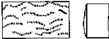
Fig. 7.2 : Hammer Dressed Stone Surface
